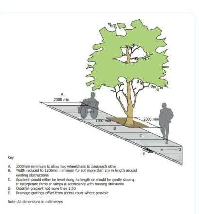
Figure 11: Figure 1.6 from Building for Everyone: A Universal Design Approach - Booklet 1, indicating absolute minimum footpath widths allowable over a short section
