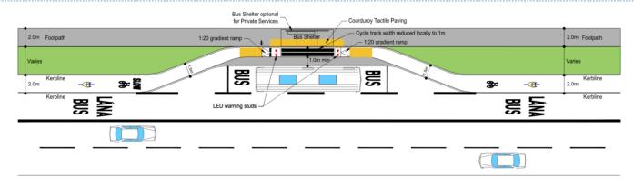
Figure 38: Lay-by Bus Stop Landing Zone Arrangement (Private Service Coaches)
