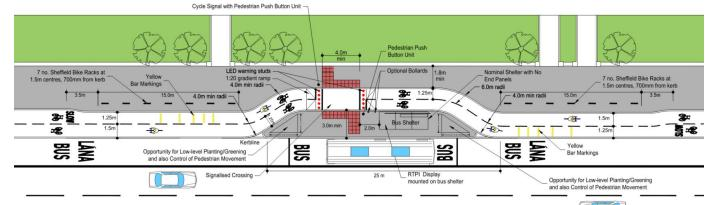
Figure 34a: Island Bus Stop Arrangement with 2-way cycle track
