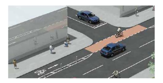
Figure 32: On-Road Cycle Lane Priority Junction Treatment
