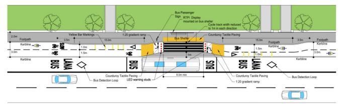
Figure 37: Shared Bus Stop Landing Zone Arrangement (Two-way cycle track)
