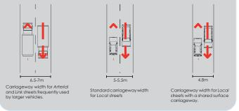
Figure 6: Extract from revised DMURS illustrating permitted lane widths
