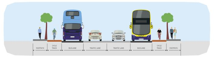
Figure 1: Optimum CBC Cross-Section
