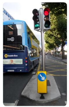
Figure 2: Signal Controlled Bus Priority
