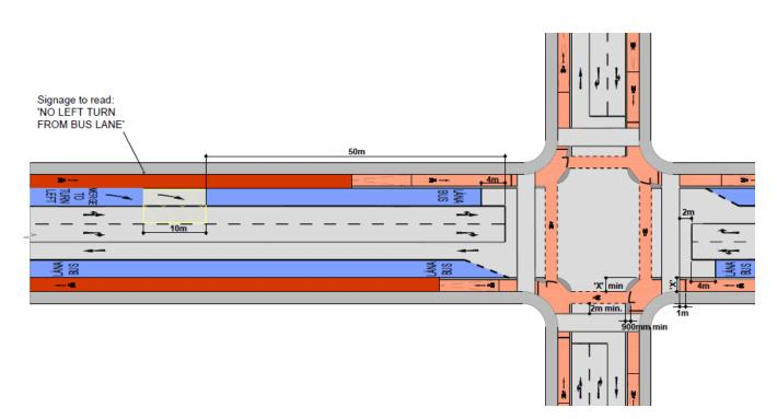
Figure 19: Example of location-specific Road Markings in advance of Bus Priority Traffic Signals
