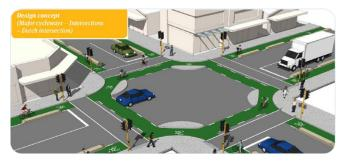
Figure 16: Key Infrastructure Elements of Protected Junction
